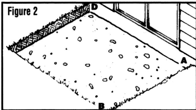
The actual excavation depth is determined by the following factors; base depth, paver thickness, sand depth, and desired finish level (see figure 1). Figure 2 shows the patio area after excavation. Locate points A, B, C & D with 3/8" diam. nails. Check that AD=BC and BA=CD at the same time AC=DB. This ensures a true rectangular patio that is perpendicular to your house. A string run from A to B to C to D can serve as a visual guide.
