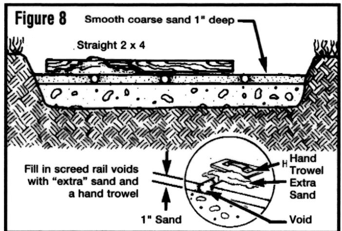
Start laying the pavers from the house out. Complete the laying process with whole pavers only. Alternate between screeding sand and laying pavers until the entire project is complete. As you lay the pavers, make sure the seams are true and square from row to row; or row to every other row, depending on the pattern you have selected.
