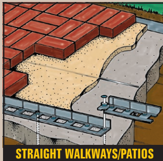
TYPICAL PAVER INSTALLATION CROSS-SECTION
